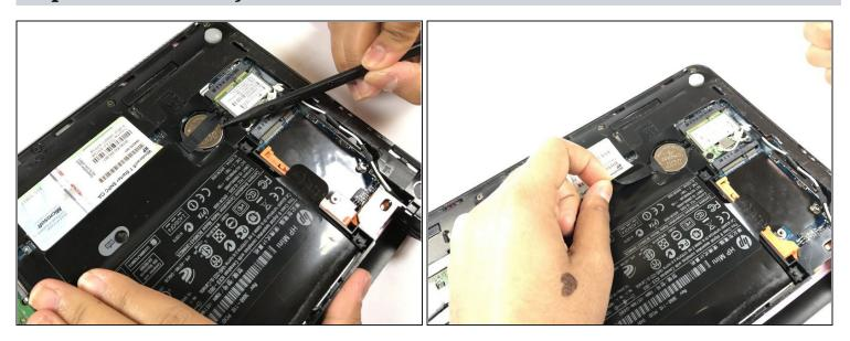
• Simply pull the small black ribbon off of the battery with either your finger or a pair of <u>tweezers</u>.
