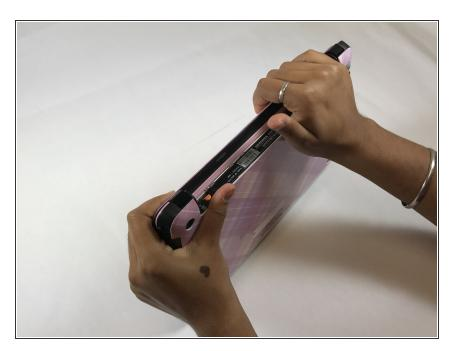
Remove the battery from the device.
