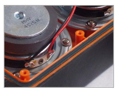
Inspect the gasket around the perimeter of the frame. Remove the gasket using your fingers or needle nose pliers.
