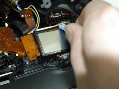
Pry off the small metal brace holding the LCD screen. (Push forward and slide toward the center)
