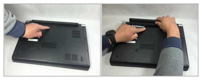
Slide the battery release slider all the way to the right and push the battery straight out of the back of the computer
