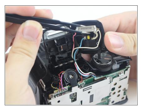
• Using a pair of ESD-safe tweezers, remove the flashbulb.
