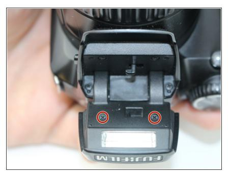
• Remove the two 5.0 mm JIS #000 screws highlighted in the picture.
