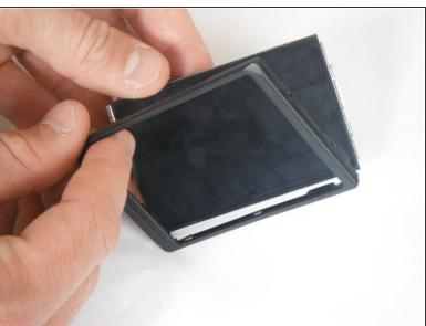
Slide the wide plastic opening tool underneath the crack of the side of the face and separate the components.
