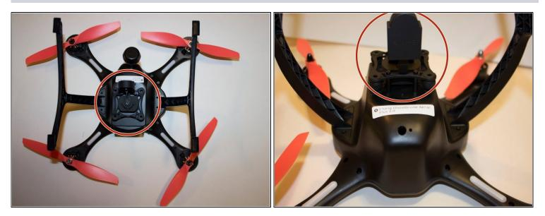
• Turn the drone on its back and identify the gimbal.
