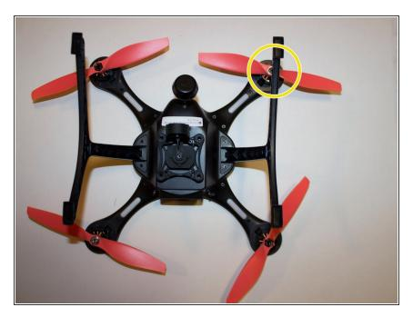
Turn the drone on its back and identify the propeller that needs replacing.
