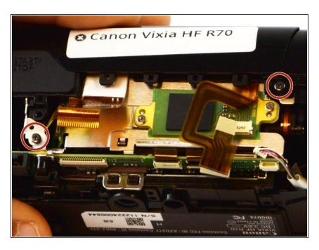
Locate and remove the two 3mm
