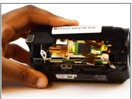
Disconnect the four ZIF connectors by grasping the connector firmly and pulling gently.
