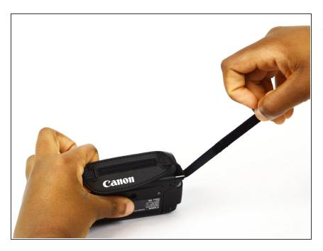
Gently pull on the loose end to separate the Velcro.
