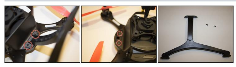
Remove the four screws attaching the legs to the drone using a Hex 2.0 screwdriver.
