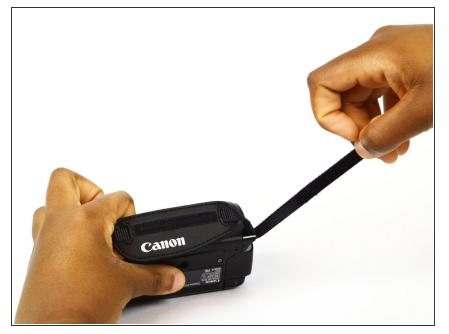
• Gently pull on the loose end to separate the Velcro.
