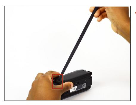
Pull the strap through the slot on the left side of the camcorder.
