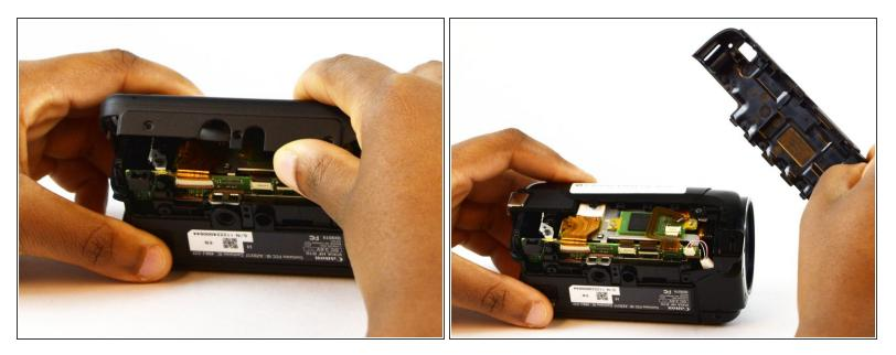
• Gently remove the side panel by pushing it up from the bottom.
