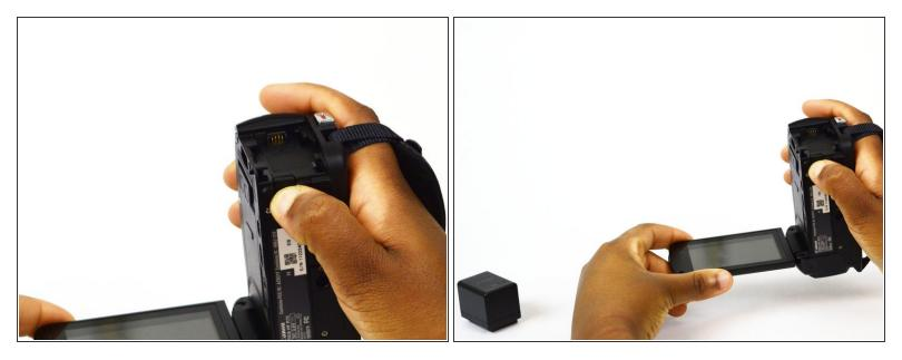
• While holding down the latch, remove the battery by pulling it out of the device.
