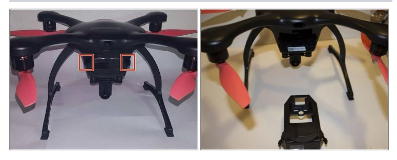
While the drone is facing forward, pinch the two tabs on the capsule, and pull it forward.
