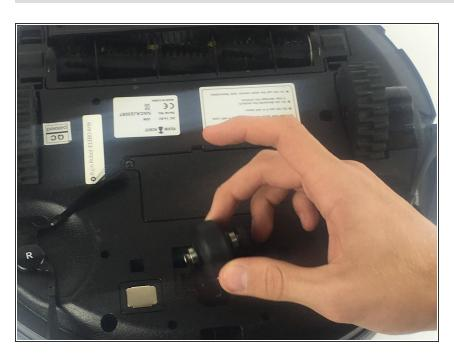
Remove the front wheel and clean its axle of any hair and debris.
