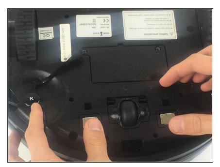
Locate the panel which covers the wheel on the back of the Yujin Robot iCLEBO Arte.
