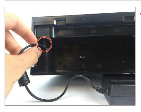
Remove the long cable from inside the base and gently pull the connector from the base.
