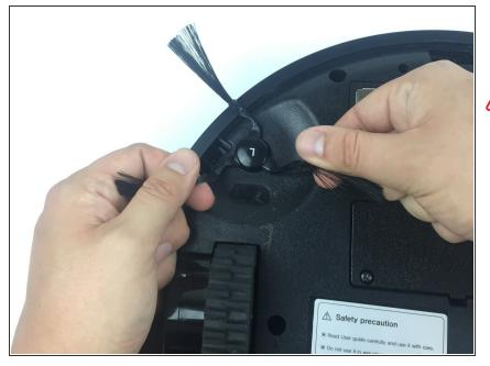
• Grab the sweeper and carefully pry the side sweeper from the chassis.
