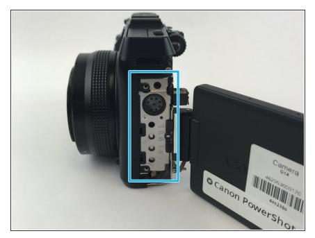
Remove the side panel covering the speaker by gently pulling it away from the camera. You can also use spudgers to create a lever to help remove the panel.
