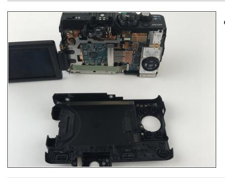
Remove the back casing by gently pulling. You could also use spudger to create a lever to help pry it off.
