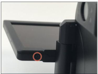
• Remove the screws on the side of the screen casing next to the hinge on the camera.
