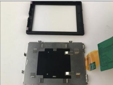
• Completely remove the casing from the screen and replace.
