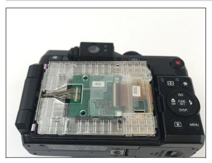
Remove the back side of the screen casing. When removing this back casing there will be a clear plastic piece inside, remove this as well. If this is the piece you are servicing, replace it and skip to the conclusion of this guide.
