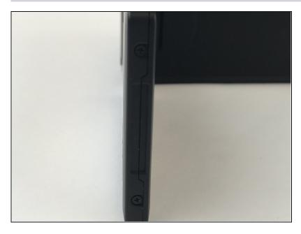
Remove the screws on the outside of the screen case shown in the photo.
