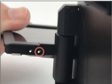
• With the plastic piece removed, locate the screws on the outside and inside of the casing shown in the photos. Remove these screws.
