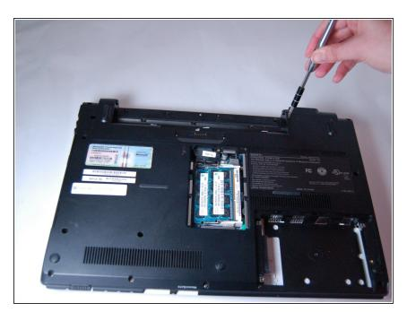
Using a Phillips #0 screwdriver, remove all twelve screws (Length: 7.7 mm) that hold the bottom cover.
