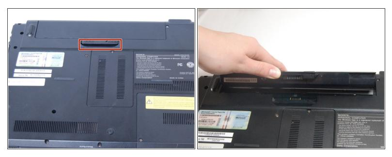
Use fingernail or plastic tool to lift the battery. Rotate the battery up and away to remove from the laptop.
