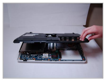
• Lift and remove the back cover.
