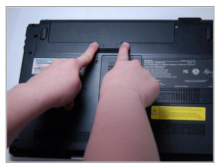
• Slide the two latches towards the center of the laptop in order to release the battery.
