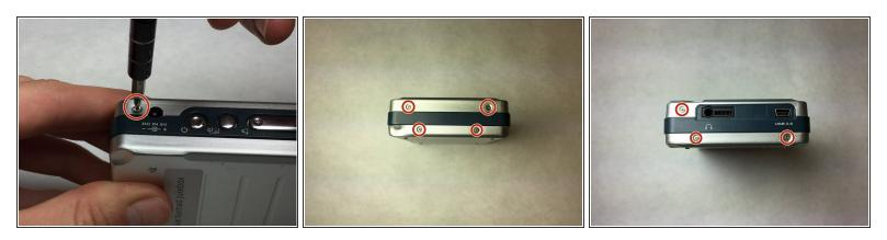
• Use a J0 screwdriver to remove the eight 3.5mm screws.
