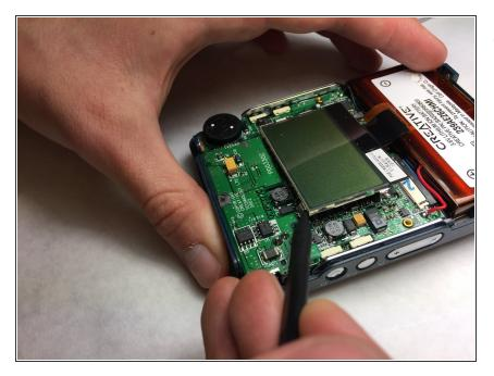
Using the spudger tool, gently pry up the corners of the display screen to remove it.
