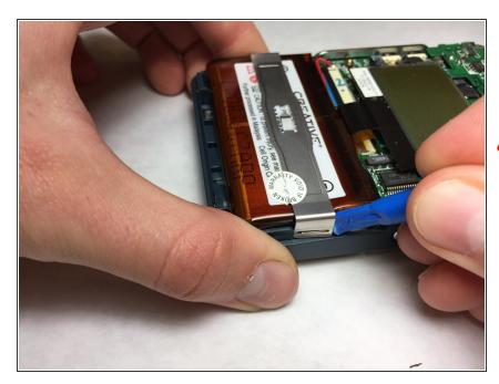
Using the plastic opening tool to pop the metal tab holding the battery in place.
