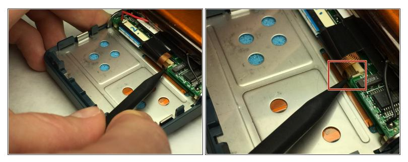
Use the spudger tool to unclip the screens wiring pigtail clipped into the motherboard.
