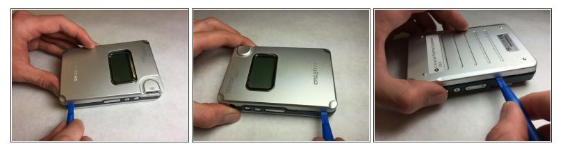
• Use the plastic opening tool to open the top cover by carefully prying at each corner.
