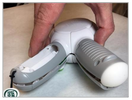
• Slightly lift up on the back cover until the handle covers are free to rotate.
