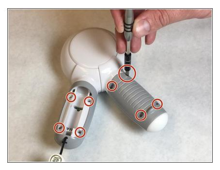
Use the screwdriver to remove the eight 8.7mm PH1 Phillips head screws.
