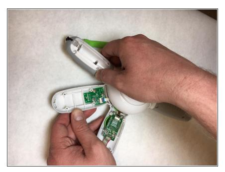
Slide the the side of the handle facing you to the left to reveal the "A" and "B" button circuit board.
