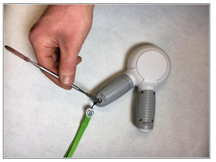
• Use the Metal Spudger to push the release clip on the battery cover.
