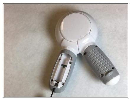
• The battery holder is now visible with the removal of the cover.
