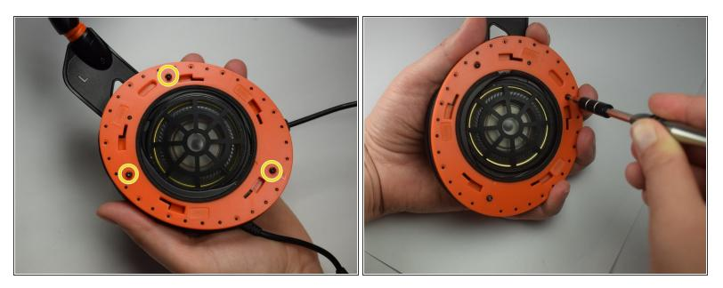
• Using the Phillips #0 screwdriver, remove the 6.0 mm screws on the orange plate.
