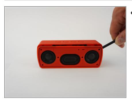
Insert the Spudger between the corners of base and the face of the speaker to open the device. The screw on the upper right corner may be difficult to take out. If you cannot take it out with a screwdriver, using force to pull the face of the speaker apart may break the plastic that surrounds the screw.
