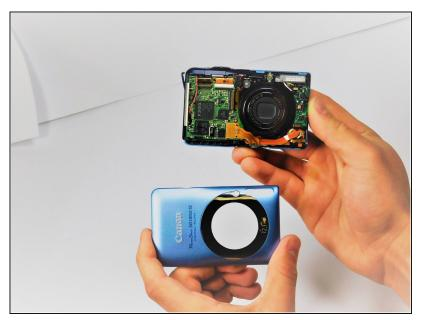
Once the front shell of the camera is removed the back shell should slide off just the same.
