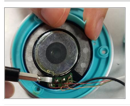
Once the loose wire or wires are located on the back of the speaker, use a soldering iron to attach the loose wire back onto the speaker.
