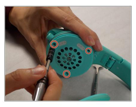
Use a Phillips #2 screwdriver to unscrew the three 5mm screws that secure the speaker cover.
