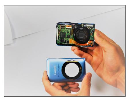
Once the front shell of the camera is removed the back shell should slide off just the same.
