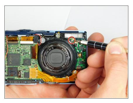
Remove a 3mm J00 screw from behind wires under the flash.
