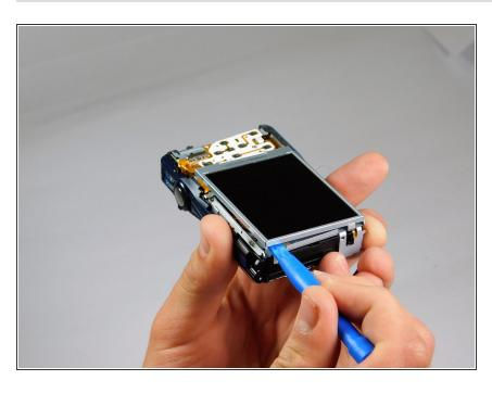
Use plastic opening tool to remove the screen to gain access to the screws to remove the Flash Assembly.
