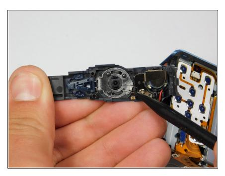
Insert Heavy-Duty Spudger under shutter button to release shutter button.
