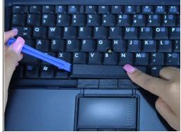
Place a plastic opening tool, under the edge of the space bar and gently pry up to release the spacebar.
