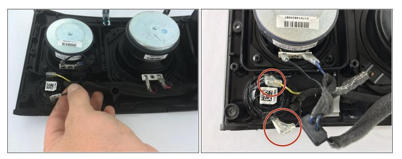
• Remove wires connected to the Tweeter.
