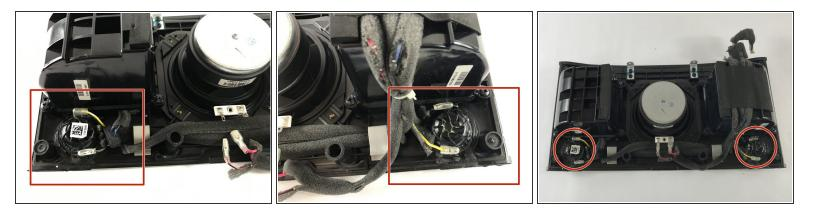
• Locate the Tweeters on the back of the front panel assembly.
