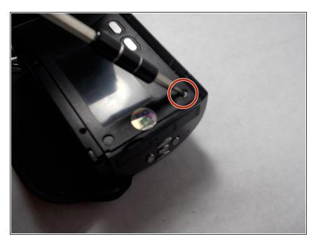
Remove the 1 mm screw shown in the picture
