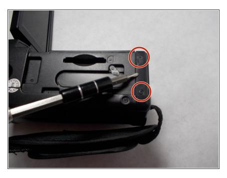
Remove the 1mm screws above and below the screwdriver.
