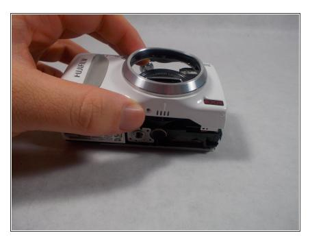
With the the camera on a flat surface with the LCD monitor on the surface, lift the front panel of the camera gently up.
