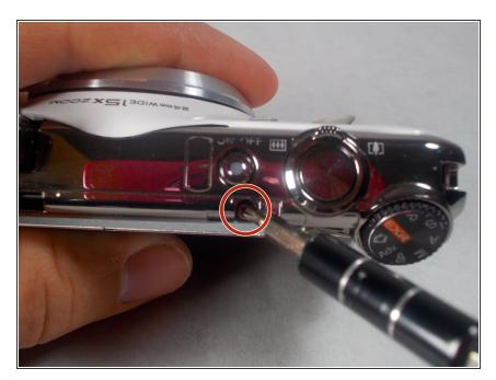
Remove the 5mm Phillips #1 screw at the top of the camera.
