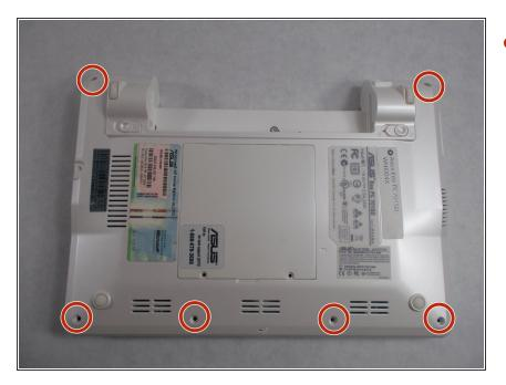
Remove all six 3.4mm Phillips #1 screws marked with red circles.
