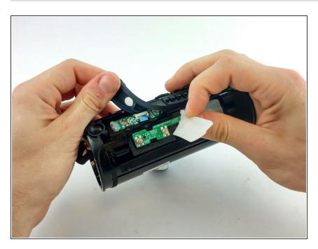
Remove the silicone button cover to expose the power chip.
