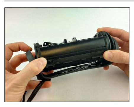
Carefully remove outer housing to expose the inner components of the speaker.
