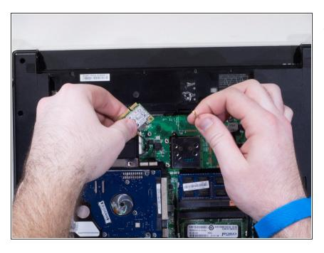
Once the screws are removed, there will be 2 wires attached to the card.
