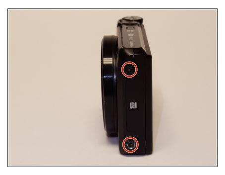
Turn camera on its left side and remove the two 40mm JIS screws by using a JIS J000 screwdriver.
