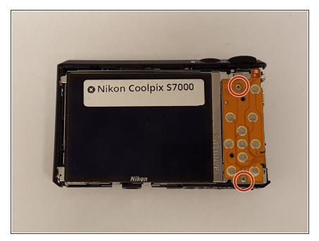
Remove the two 20mm JIS screws using a JIS J000 screwdriver. They are responsible for keeping the keypad in place.
