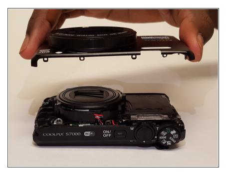
Carefully remove front cover of the camera.
