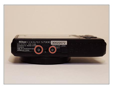
Turn the camera upside down and remove the two 40mm JIS screws by using a JIS J000 screwdriver.
