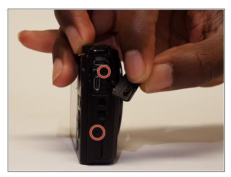
Turn the camera on its right side and remove the two 40mm
