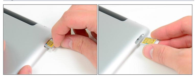
• Pull the SIM tray out of its slot and remove it from the iPad.
