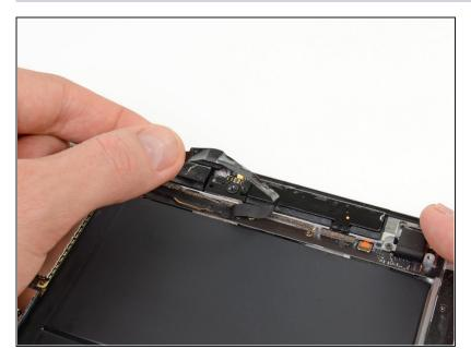
• Peel back and remove the adhesive tape covering the headphone jack assembly.
