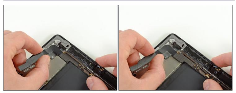
• Holding onto the ribbon cable of the headphone jack assembly, carefully pull the assembly parallel to the iPad, toward the bottom of the device.
