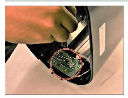
Locate the circuit board inside front cover.
