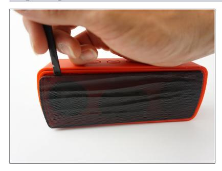
Insert the Spudger between the grated panel and the base of the speaker.
