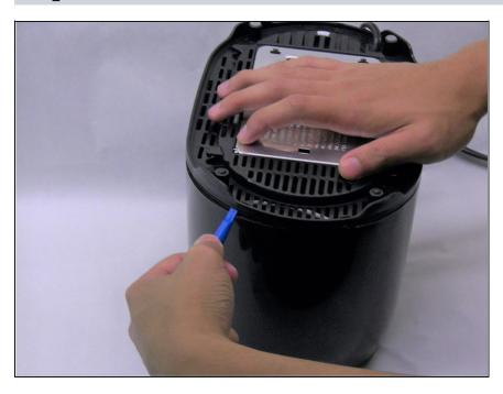
Detach the bottom from the front cover using the plastic opening tool.
