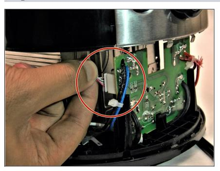
Detach the bundled cable connector from the toaster by carefully pulling it away from the circuit board.
