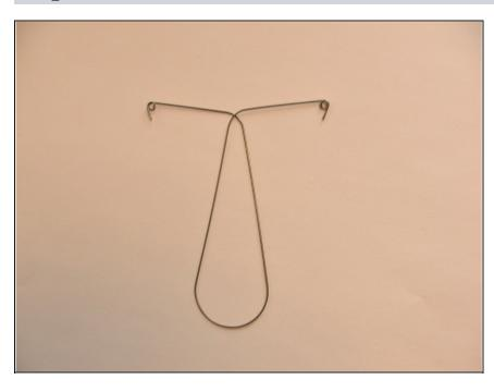
Remove the old spring from the toaster unit to insert the new one.
