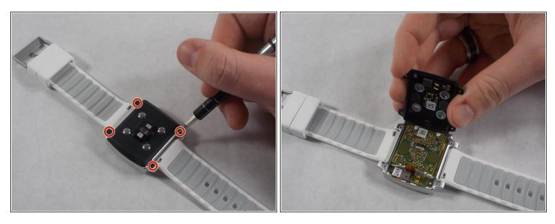
Remove the four base screws using a size 2 TORX screwdriver to separate the back plate from the frame.
