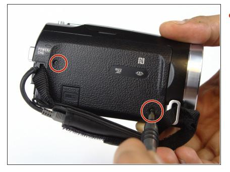
Turn the camera to the handgrip side and unscrew two of the 5.5mm JIS #00 head screws using the JIS #00 head screwdriver.
