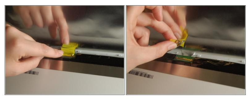
• Pull off the tape and disconnect the display cable connector by gently sliding up to remove it from its socket.
