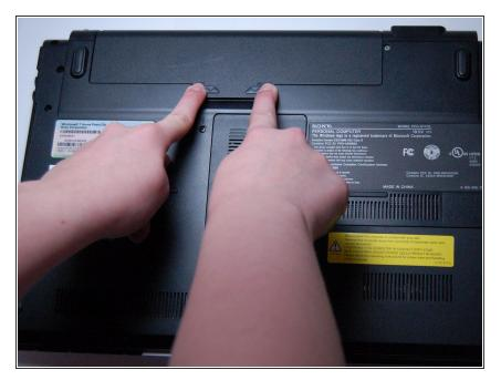
• Slide both latches towards the center of the battery to release.
