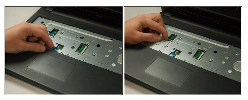
Unplug the touch pad cables located on the palm rest.
