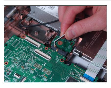
Loosen the cables on the antenna.
