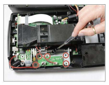
Next, remove the 5 9mm x 5mm screws from the circled spots with a Phillips J1 screwdriver.
