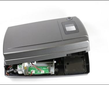
■ To start, open the device by removing the 5, 5mm x 9mm screws, with a Phillips J1 screwdriver.
