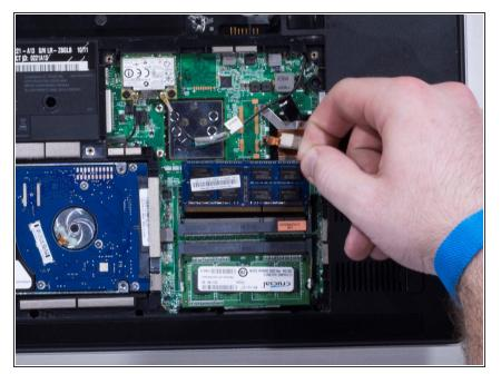
Once freed from the brackets, the RAM can now be easily pulled out of its slot.
