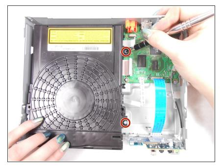
Unscrew the two 8mm Philips head screws securing the disc assembly to the main casing.
