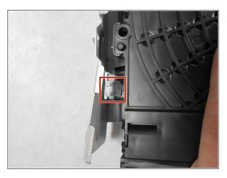
Pull the disc assembly out from under the metal tabs on the main casing.
