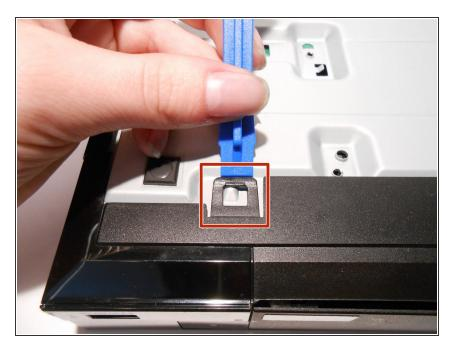
Using an opening tool lift up the tabs located on the bottom of the plastic front cover.
