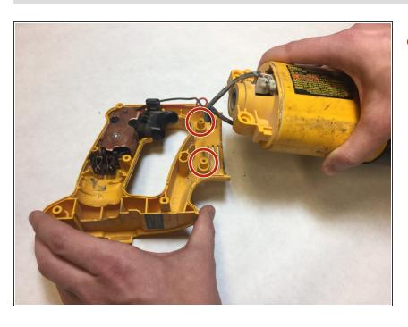
Lift the mechanical device off the pins of the clam shell.
