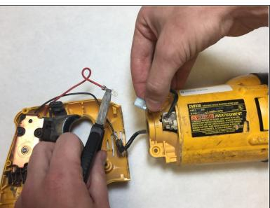
Remove the red and black trigger wires from the brush leads with the pliers.
