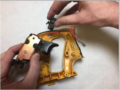
Remove the VSR trigger and the lock button.
