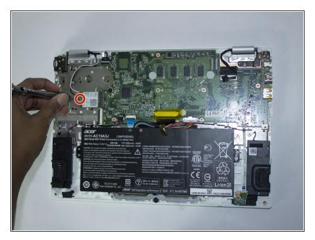
Remove the single 2.85 mm Phillips #1 screw that secures the wireless card.
