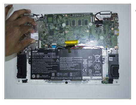
Carefully slide the wireless card out of its socket on the motherboard.
