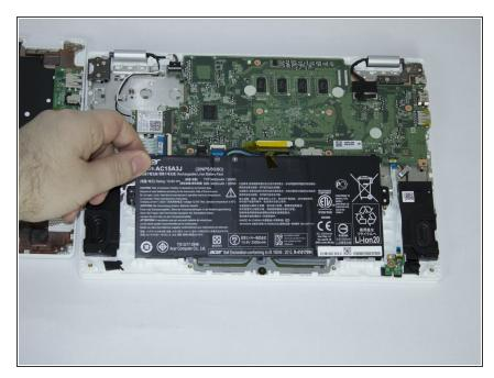
Remove the battery by pulling upwards.
